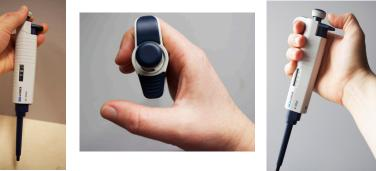
5. Putting a tip on your micropipette involves choosing the right size tip. The picture below shows the different sizes of ASSET pipettes and the tips that go with each. Usually, the larger the volume, the larger the tip. Logically, the P10 uses the P10 tips, the P1000 uses the P1000 tips. However, the P200 tips will fit the P20, P200 and 8-channel pipette.
