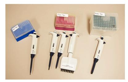
6. Use a steady hand to hold your pipette, open the tip box and firmly press the pipette into the tip. **DO NOT** tighten the tip with your fingers as this increases the likelihood of contamination. If you press down firmly while the tip is in the box, you will properly tighten the tip. Pull your pipette straight out of the box and put the lid back on the tips to prevent contamination of your tip box. **ALWAYS PUT A TIP ON YOUR PIPETTE BEFORE USE!**
