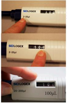
1. Use a micropipette when you are working with small quantities of liquids. Before using a pipette you should always know the volume you need and what pipette is the appropriate size for your use. The volume minimum and maximum will be listed on the side of the pipette. In the image to the left, the minimum amount is  $2\mu$ L and the maximum amount  $20\mu$ L.
