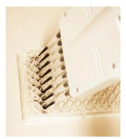
4. Once you have successfully filled all 8 pipette tips, transfer the liquid to the appropriate row in your 96-well plate. Press down to STOP ONE to release the liquid and then to STOP TWO to ensure that all the liquid has been released from the tips. Pull the tips out of the wells **BEFORE** releasing the plunger, otherwise you will draw back up the liquid you just expelled.
